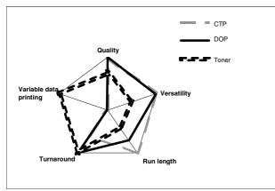
Figure 4. Relative strengths of toner, CTP and DOP
