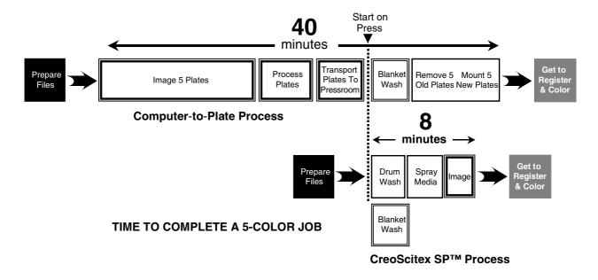
Figure 6. SP means shorter cycle time and reduced number of handoffs
