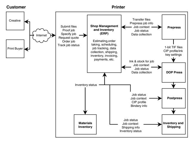
Figure 5. Integrated workflow for profitability
